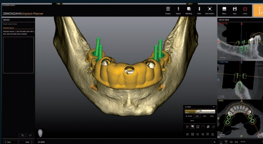
Fig. 3: The finished virtual model of the surgical guide with apertures to check for proper intraoral seating. The data can now be exported to produce the surgical guide.
